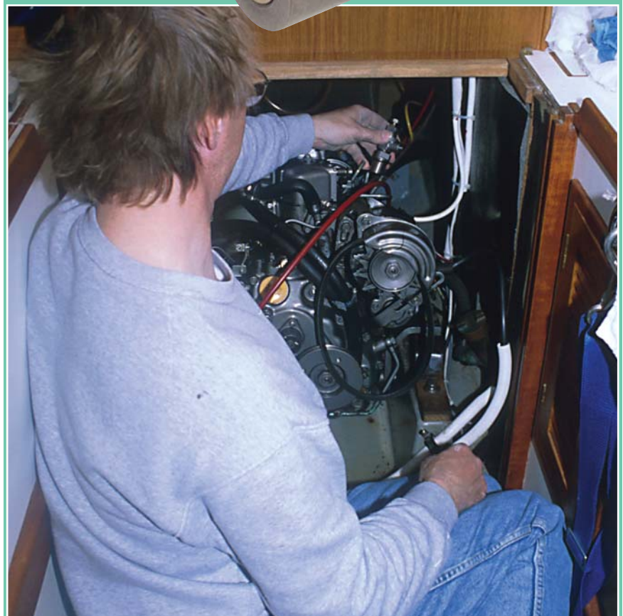
Keeping your engine running at peak performance requires routine maintenance. Top: Injectors are simple to replace; this one's from Yanmar
