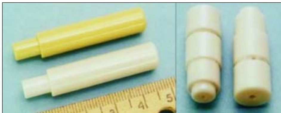
Zirconia fuel injector components are replacing metal ones, eliminating some of the problems associated with the use of low-sulfur diesel fuel.
